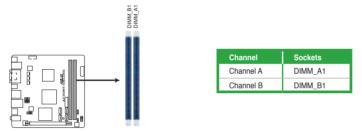
AT3IONT-I SERIES 240-pin DDR3 DIMM sockets
