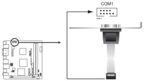
AT3IONT-I SERIES Serial port (COM1) connector
