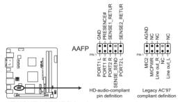
AT3IONT-I SERIES Analog front panel connector
